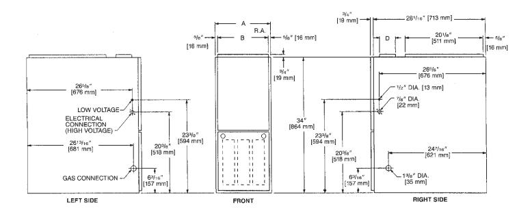
TABLE 1. DIMENSIONS AND CLEARANCE TO COMBUSTIBLE MATERIAL (INCHES) [mm]
